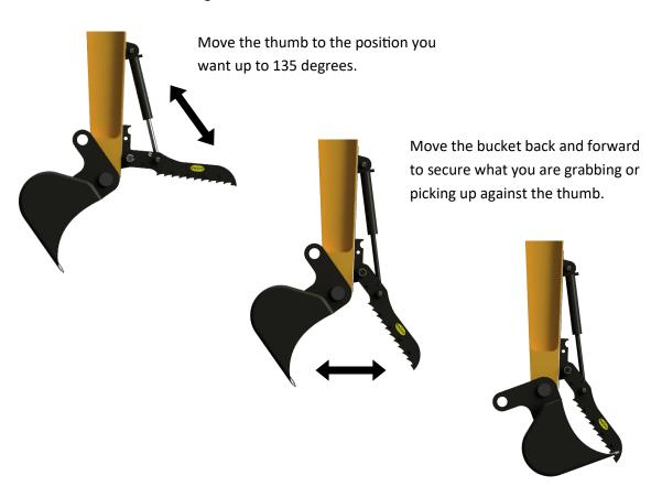
When your KNAPP Hydraulic Thumb is not in use, it tucks away. A separate position pin can be used to secure it in place. If you do not need to use thumb for a long period of time, or you need to reduce weight on the dipper arm, you can unpin the thumb and remove it from its backing plate.
