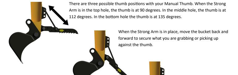
When your KNAPP Manual Thumb is not in use, it tucks away and is pinned in place. As the Strong Arm is a separate part, it is stored in the excavator cab when the thumb is tucked up. If you do not need to use the thumb for a long period of time, or you need to reduce weight on the dipper arm, you can unpin the thumb and remove it from its backing plate.
